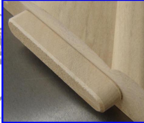
A pre-set amount of stock is removed from each end of the part during the machining process. If an accurate cut-off saw is not available, consider one of the optional sizing fences.
